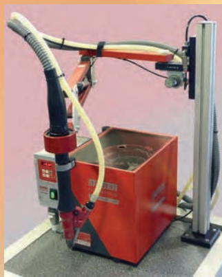
Hand screwdriver with automatic feeder
