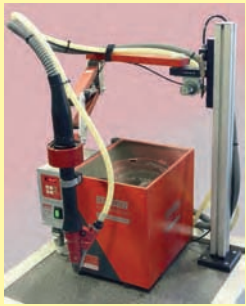
Feeding and Control Unit HSE
