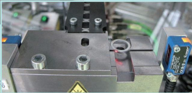
Sorting rail with delivery point for sealing rings
