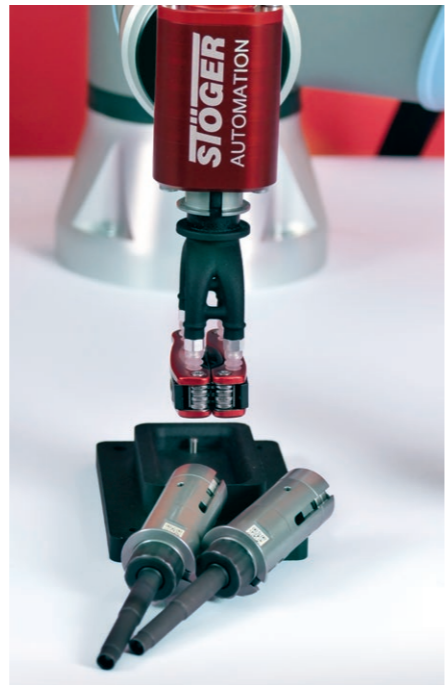
Gripper and two screwing tools. Attached to the tools are the scan codes for the encoder.
